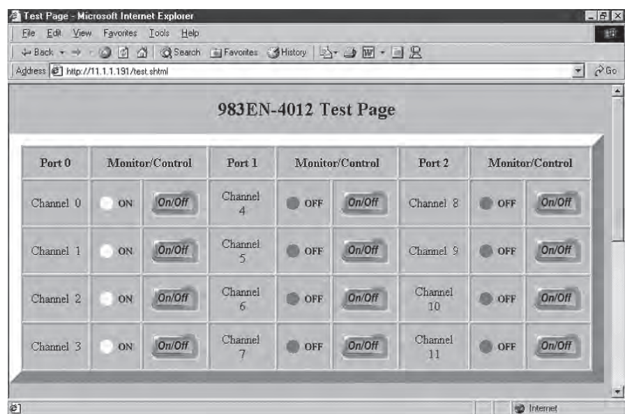
Figure 3: A test page is also accessible with your web browser to confirm proper operation of the I/O module.
